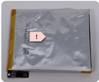
Swelling or electrolyte leakage
